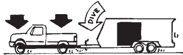
Weight distributing hitch transfers loads to frame and to both axles of tow vehicle for safer stops and smoother ride.
